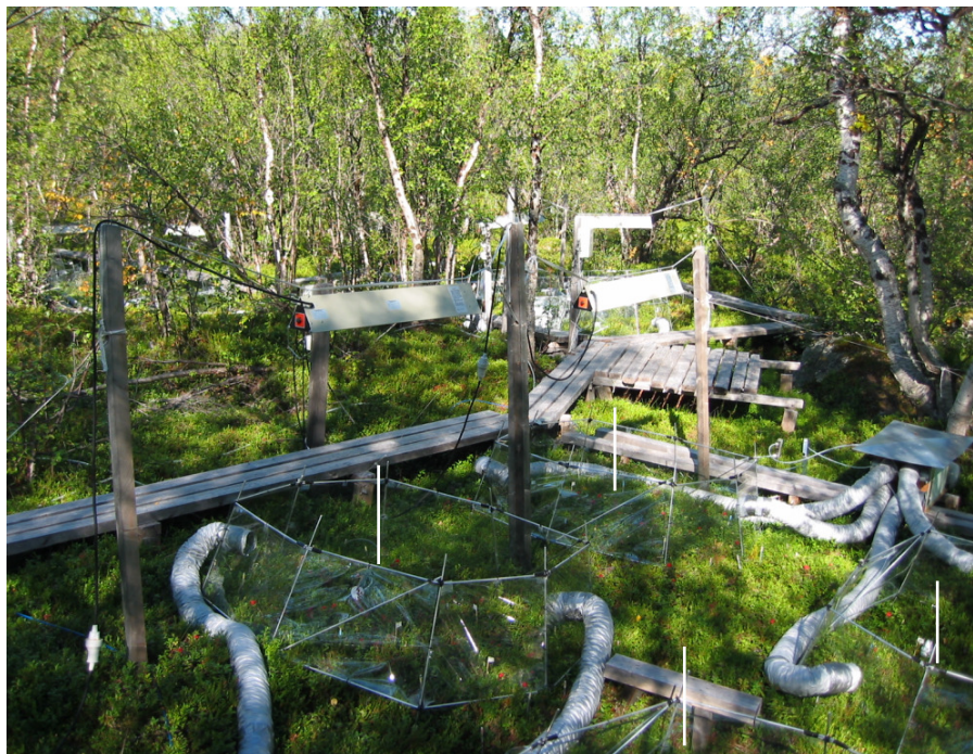
Figure 8.3. Example of factorial experiments with increased temperature (infra red lamps and soil heating cables) and increased carbon dioxide concentration at Stordalen, subarctic Sweden (experiment operated by the Ecosystems Centre at Woods Hole).
